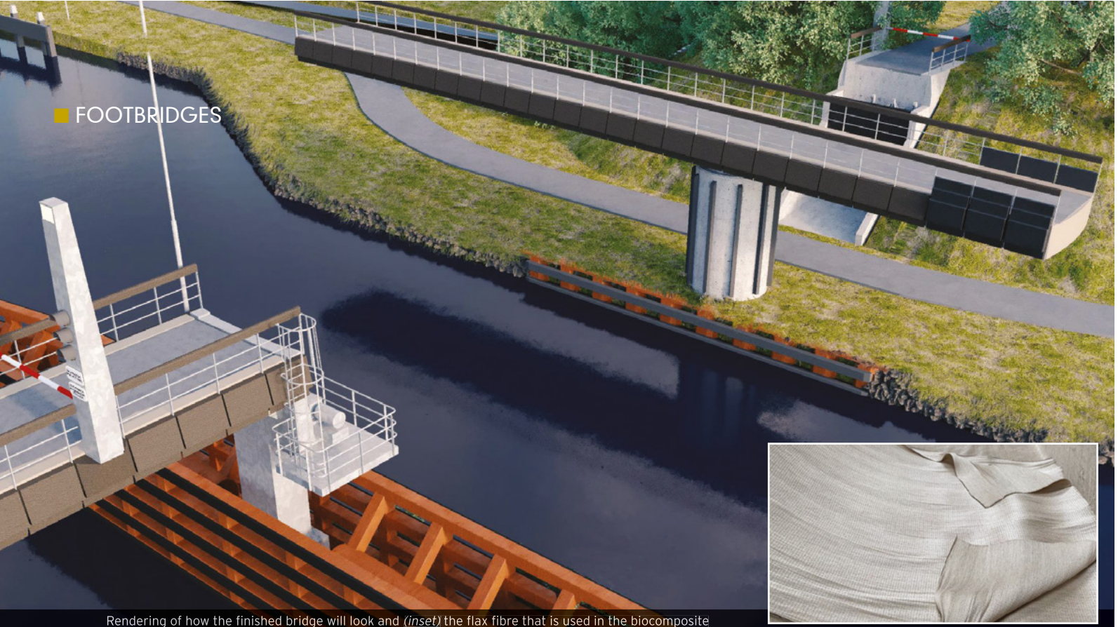
Rendering of how the finished bridge will look and (inset) the flax fibre that is used in the biocomposite
